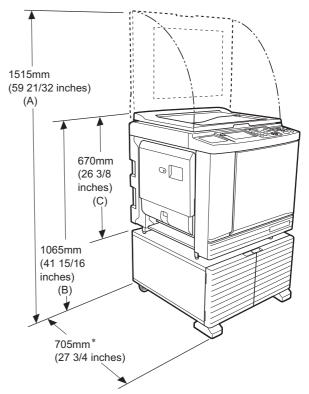
When the optional auto document feeder is installed, the values of (A) to (C) in the figure above are as follows
