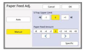
Touch [Specific] to specify [Clutch ON Timing] and [Clutch OFF Timing].
