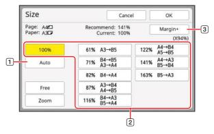
[Auto]: The size of the original is automatically enlarged or reduced according to the size of the paper on the paper feed tray.
