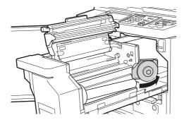
6 Remove the depleted master core.
