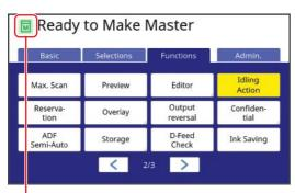
When [Idling Action] is turned on, the icon that is displayed in the message area of the master making basic screen is changed.
