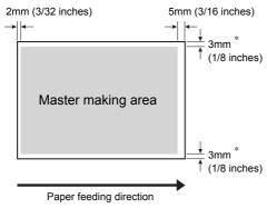
\* These values are for cases when using standard size paper. When using custom size paper, these values are 5 mm (3/16 inches).
