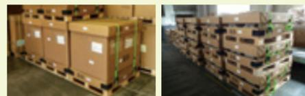
Shipping of ORPHIS printers using returnable pallets. Pallets can be folded to small size for return after shipping.
