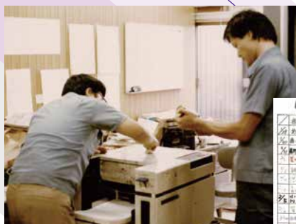
“One million page test” that was carried out in shifts by groups of two people and a progress chart on which each supervisor recorded test results
