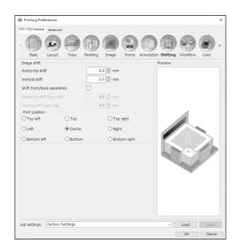
Adjusts the vertical and horizontal margins of the original images.
