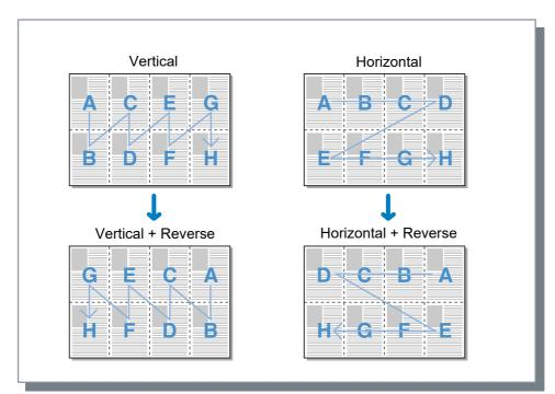
If [Multi-up (Plural)] or [Multi-up (Single)] is selected at [Imposition], set the number of pages per sheet for imposition. 2, 4, 8, or 16 pages/sheet can be selected. The default setting is 2 pages/sheet.
