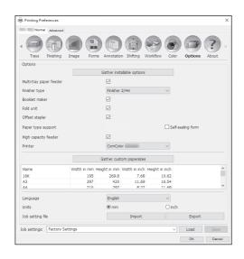
Configures optional devices connected to printers, and registers custom paper sizes in the printer driver. "Options" @p.103
