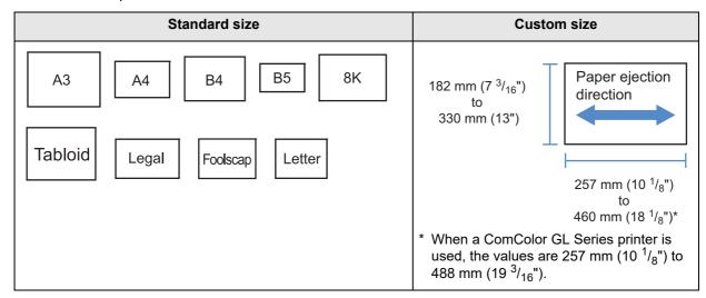
When using custom-size paper, do not allow the vertical length of the paper to be longer than the horizontal length.
